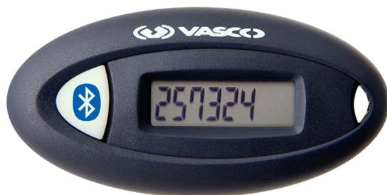
With any Bluetooth Smart Ready mobile device, the DIGIPASS GO 215 instantly creates a virtual secure channel between the back end and the device, to encrypt or decrypt server commands. The end-to-end encrypted channel introduces an unprecedented level of security, enabling organizations to instantly and securely exchange information with users and reinforce the security of their applications without requiring pairing or any additional configuration.
