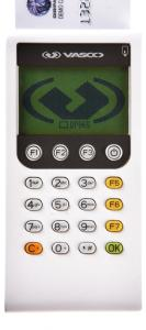
from a security point of view. DP 865 provides the secure advantage of entering the pin directly at the reader and not on the computer keyboard. Therefore, the PIN is never available on the PC platform. Similarly, smart card PIN changes can be securely performed using the DP 865 keyboard.
